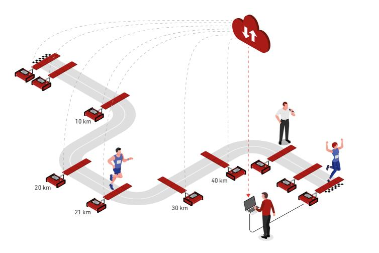
The easy and fast setup of splits is a major benefit of the RACE RESULT Passive Solution. Combining the foldable ground antennas, Ubidium and our high-quality UHF transponders provides efficient workflows, highest detection rates and live results for all participants. This way, races of any size can be timed.
