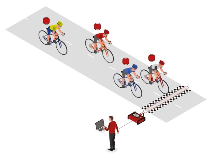
Even short time intervals in sprint finish situations are reliably timed with the Active Pro V3 transponders. Ubidium can detect the times of up to 100 active transponders per second.
